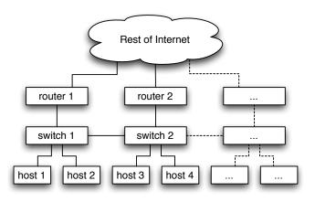
Figure 1: Components of the Anycast Cluster
